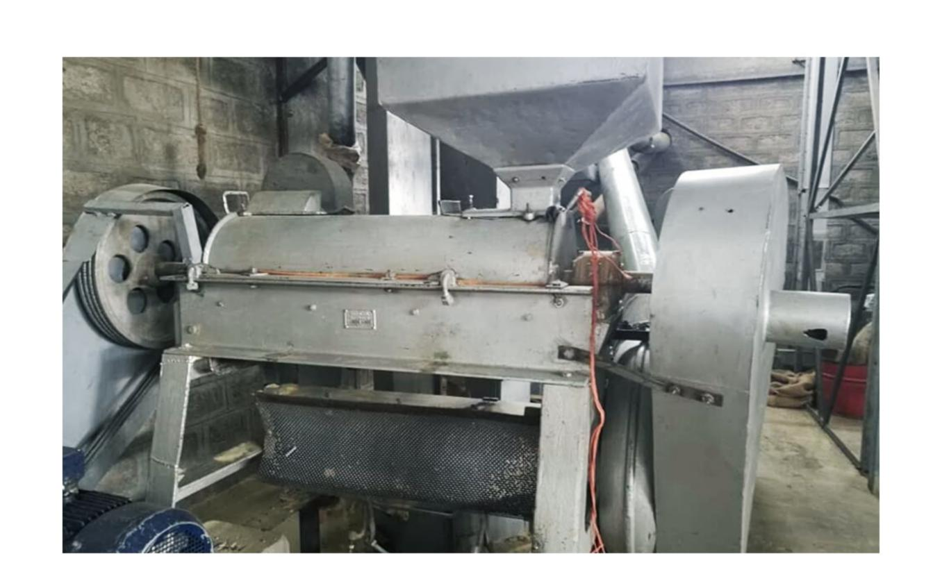
The polisher removes the silver skin of the hulled coffee, to increase the optical appearance of the grain and facilitate the optical sorting and roasting process.
