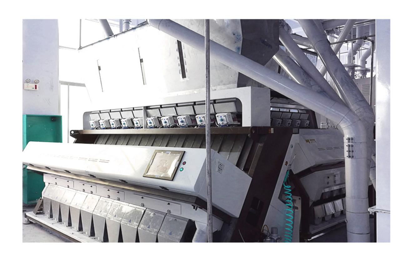
The pretreated coffee beans are irradiated by the high-definition camera inside the color sorter, and the beans of different colors will be separated by the gas generated by the high-speed spray valve. stored in separate silo. The accepted coffe bean goes directly to the next step for packaging. The color sorter can completely replace the hand-selected belt. It enables customers to save labor costs, and the product quality can be comparable to it.
