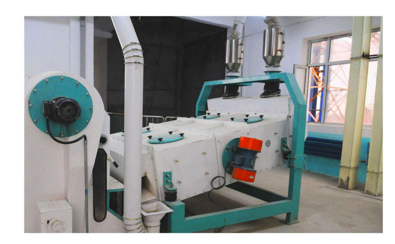
For removal of chaff, straw and other course matter complete with appropriate number and quality of screens .the destoner is to separate granular materials in dry condition e.g. stones according to specific weight in to two fractions complete liners and automatic clean out deck.
