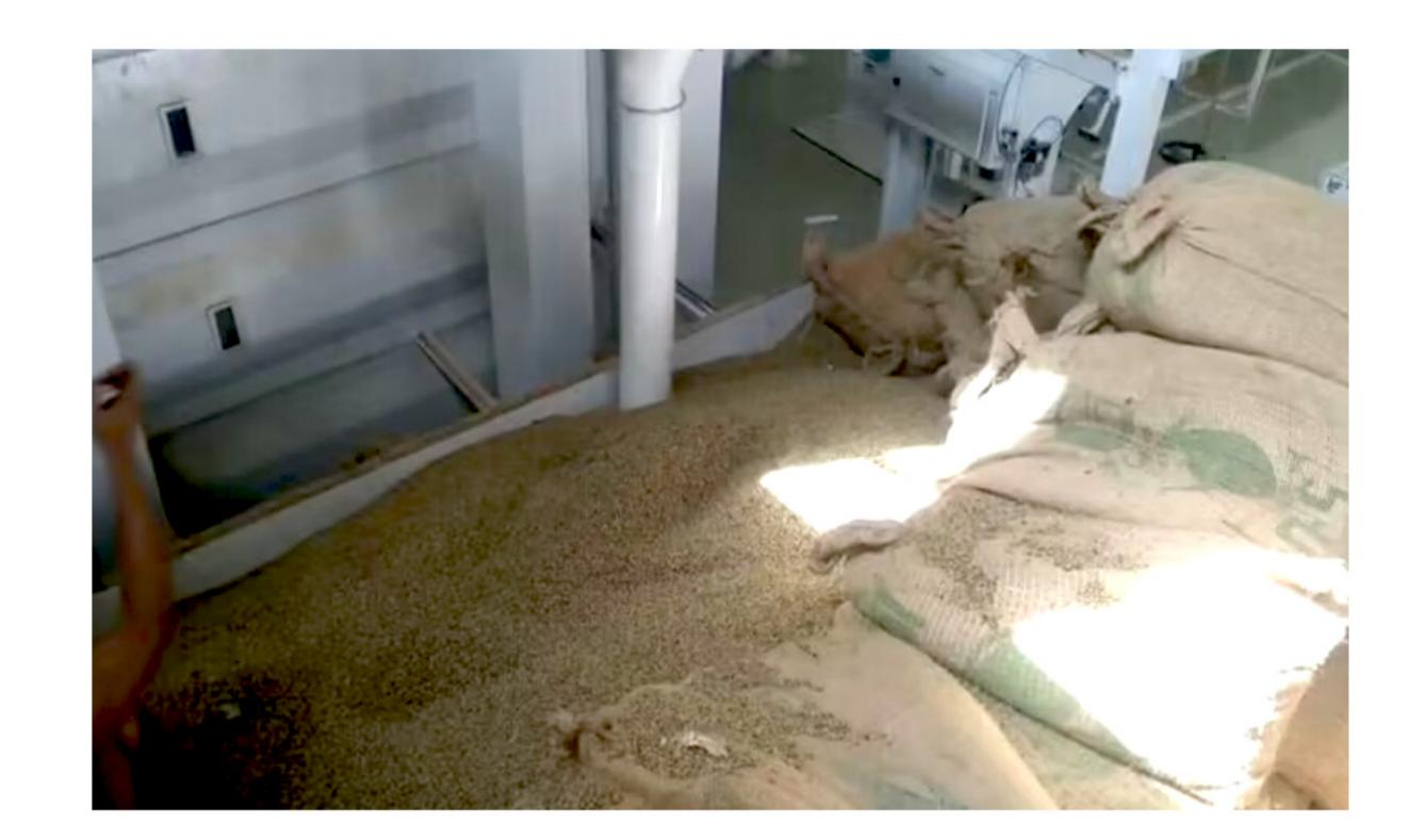
Intake hopper with supporting and steel grating. Dimensions will vary according to customer requirements and the size of the site. At the same time, we have installed a dust removal and suction hood above the hopper, so that the light impurities in the coffee beans will be eliminated at the first time and then collected into the dust collection room. Make the production environment of the workshop clean and free of dust.
